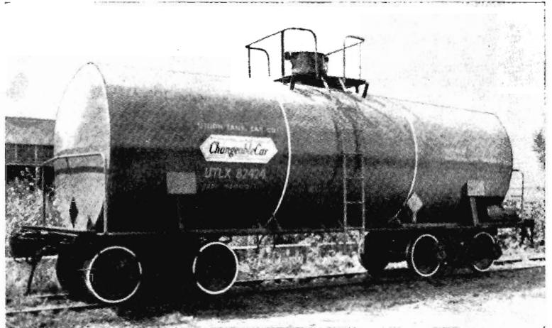
The basic elements of the *Changeable Car* consist of a keystone unit at the tanker's centre, end tubs that close the tank, and centre plate assemblies which may be altered to vary the bogie capacity.
