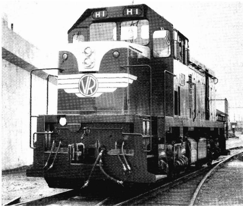
**NEW LOCO:** The first H class diesel-electric locomotive enters service near the site for the hump in the re-arranged Melbourne Yard where the locomotive will ultimately work. It is a re-classified T class loco with modified controls for hump shunting (see January *News Letter*, p. 2).
