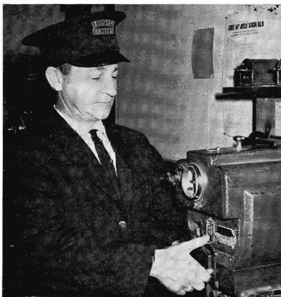
A.S.M. Illig withdrawing the staff for No. 25 rail motor.
