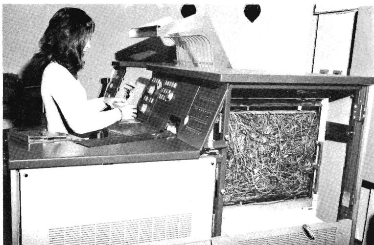
Data Processing Assistant, Michele Healy, uses the 1004 Electronic Data Processor before it was released on delivery of the new G 415 computer. Programmes for the 1004 were the maze of wires inserted on a panel (at right).
