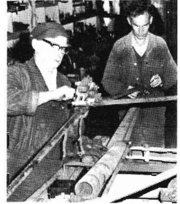
Don Mason (left) and Bill O'Loughlin go about their task of renovating a pantograph from a metropolitan train. An average of two pantographs are completely restored each week.
