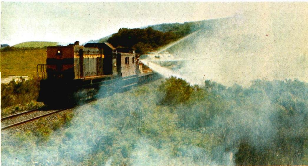
**UNDER FULL POWER** the fire attack wagon can shoot hundreds of gallons of water a minute for distances of up to 100 ft. from the line. Near the end of the project the vegetation thinned out and the steep-walled cuttings finished so that a clear view of how the train was operating could be taken.
